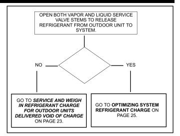
Figure 18. Outdoor Unit Factory Charge
